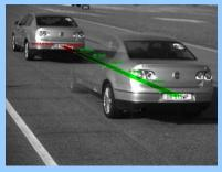
T-EXSPEED V 2.0 is the newest and most innovative digital system for detection of vehicle speed (instantaneous/average), red-light and trajectory-based violations. It does not need additional, external sensors (inductive loops, radars or lasers), as it detects the vehicle trajectory directly from images taken by high definition cameras, repeating the real time recognition process at every new video frame. It measures the speed of the vehicles up to 300 km/h.
